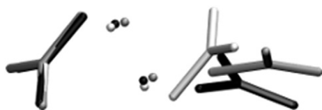
Fig. 9. Overlay comparing the structures of the calcium carbonate dimers. The original dimer before interaction with dipeptides is depicted in white, the dimer as complexed with diaspertate is gray, and the dimer complexed with diglutamate is black. The complexed dimers clearly are distorted, with respect to the original. The structures of the dipeptides were eliminated for clarity.
